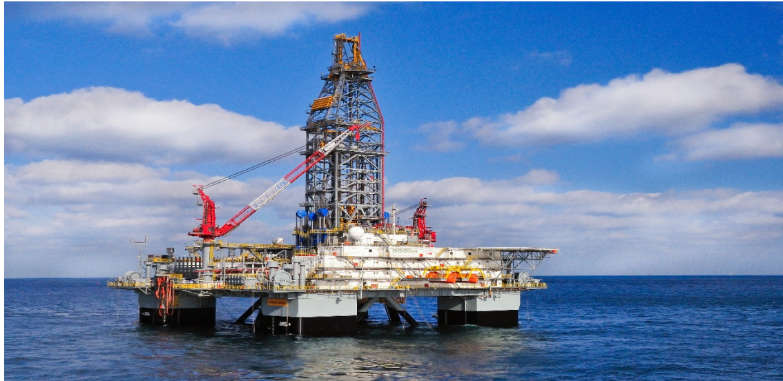
Figure 3: Enscoplac 8503 Semi-submersible 25 – This floater semi-submersible drilling rig is capable of operating in water depths up to 8,500 ft. and drilling wells up to 37,500 ft. depth. It can accommodate 150 persons.
