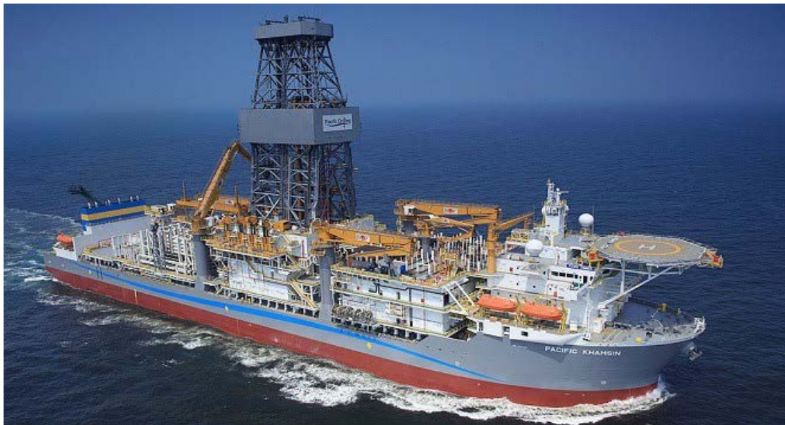
Figure 2: Pacific Khamsin Drillship 24 - This floater drillship drilling rig is capable of operating in water depths of up to 12,000 feet and drilling wells up to 40,000 feet deep. It can accommodate 200 persons.
